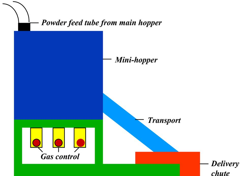
**Figure 1. Schematic of fluidized fill shoe system.**
